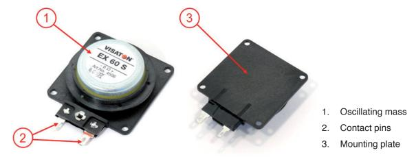
By applying a voice- or music signal to the contact pins, the oscillating mass starts shaking with the frequency of the applied signal. This oscillation is transmitted to the mounting plate and from there on to the surface the exciter sticks to. Thus, the excited surface will emit the voice- or music signal.
