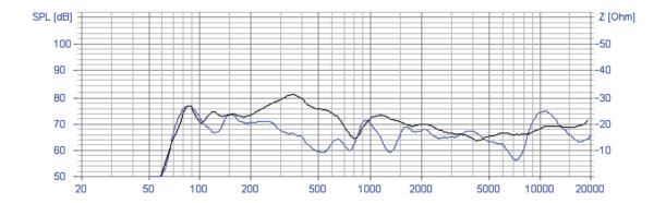
frequency response (1 W / 1 m) black = HDF board (690 x 660 x 4 mm) blue = MDF board (1200 x 800 x 19 mm)
