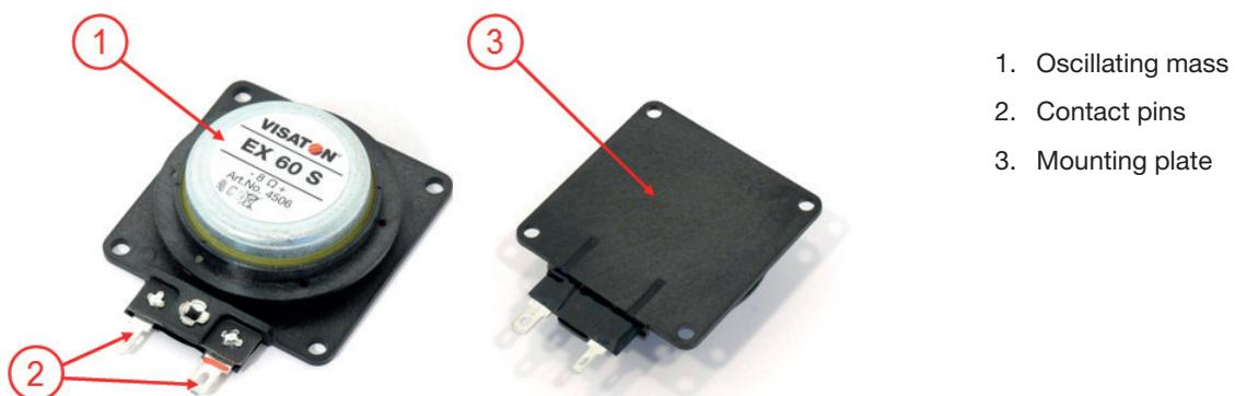
By applying a voice- or music signal to the contact pins, the oscillating mass starts shaking with the frequency of the applied signal. This oscillation is transmitted to the mounting plate and from there on to the surface the exciter sticks to. Thus, the excited surface will emit the voice- or music signal.
