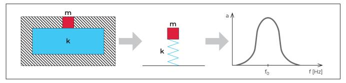
m = mass, k = spring rate, a = amplitude, f = frequency
